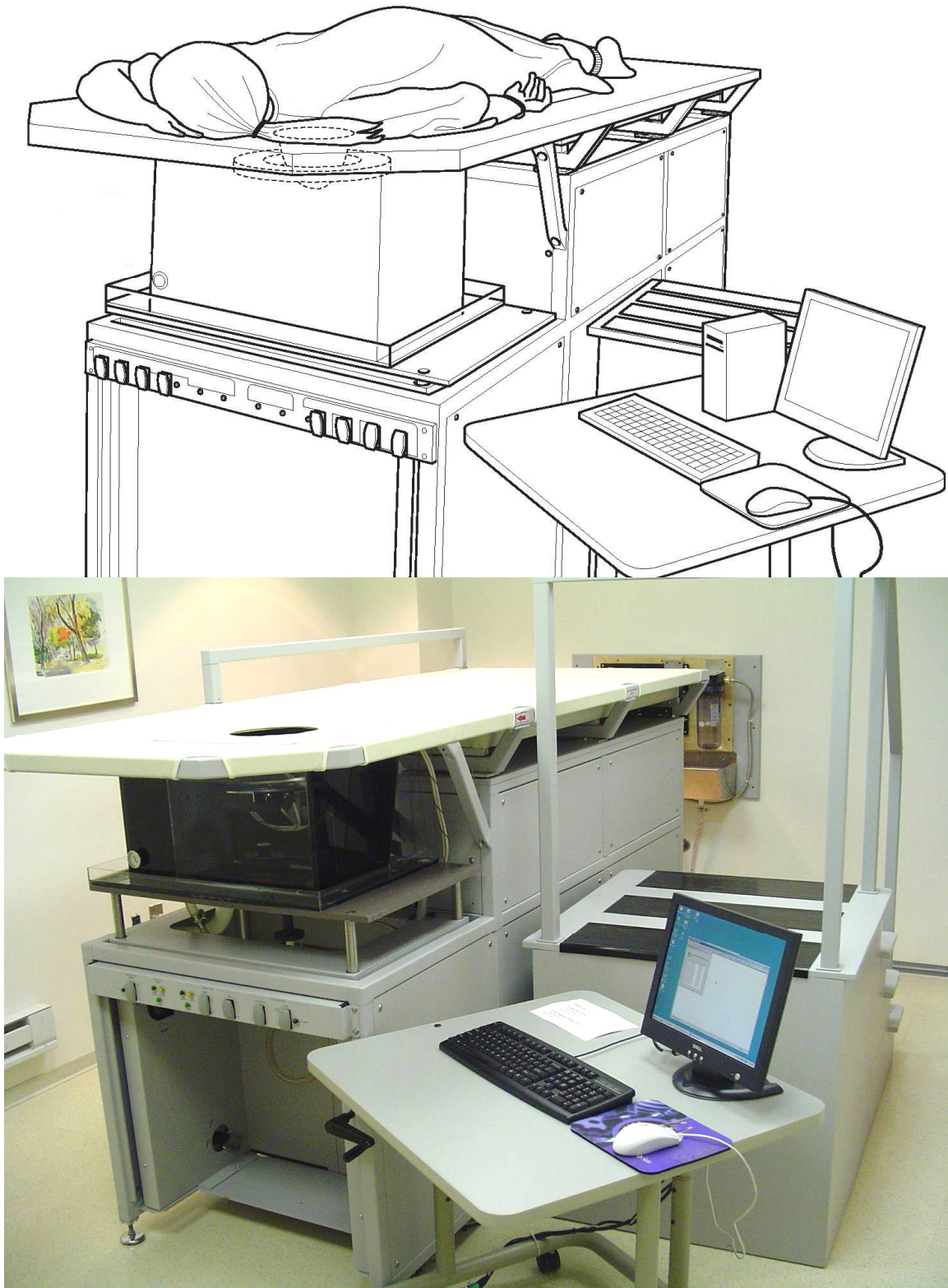
Figure 2-2 - (Top) Schematic diagram of the UST prototype showing patient positioning (Bottom) Actual UST prototype at the Karmanos Cancer Institute in Detroit, MI.
